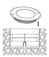
5) Use fixing SS bolts (1) to fix the head to the base
