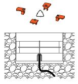
3)Connect (5) to the power and ensure no cable lengths are cut on the entry cable. Cable must be fully sealed in a Gel type connector block below the fitting. Place the probe (5) into the Housing (8) using parts (3&4).
