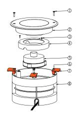
1) Core Drill a hole in the ground. Insert base (8) into said hole with concrete/Silicone . Ensure part 8 is sat horizontally. With fixing tabs (7) above the surface.
