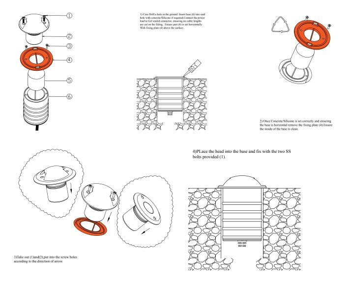
Follow installation instructions carefully. Ensure all below ground termination is totally sealed. Do not shorten the cable lengths provided on the fixture. Ensure all power is Off during installation until circuit is complete.
