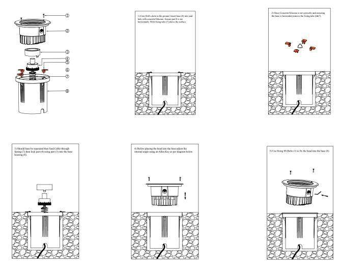
Follow installation instructions carefully. Ensure all below ground termination is totally sealed. Do not shorten the cable lengths provided on the fixture. Ensure all power is Off during installation until circuit is complete.
